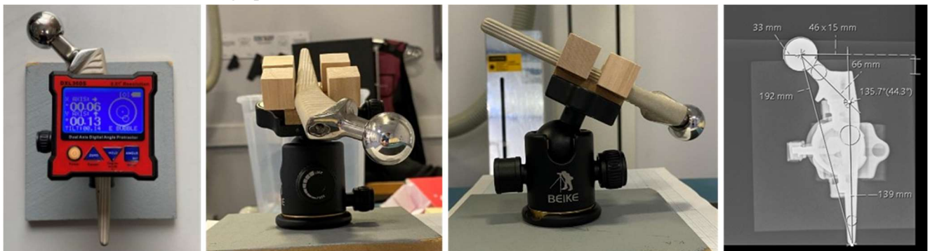
Figure 6 – Left, Gimbal setup. CORAIL stem mounted on a gimbal to allow orientation and a dual-axis inclinometer to accurately control orientation. Right, radiographic features measured from an in vivo radiograph using NIPACS.
